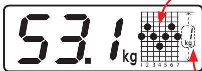
Every time that you weigh yourself, your weight is automatically stored and displayed on the graph. The graph can display up to seven different weighings.
